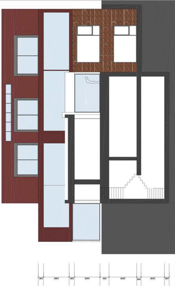
Elevation EE - sectional-elevation through garden living room looking back towards main house
